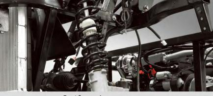
Front Suspension A MacPherson Strut type suspension ensures the best ride of all the competition while providing the driver excellent road-feel and control.
