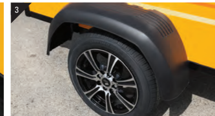
3 Fenders to protect cargo from road dust and other debris
