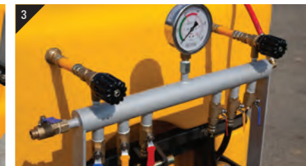
3 Distributor which can be conveniently controlled from the driver's seat
