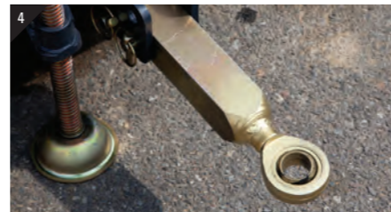
4 Equipped with a link for easy attachment to and removal from tractor
