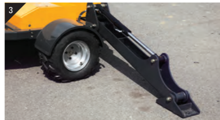
3 Folding hydraulic support to fix the lift body in place
