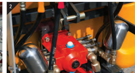
2 Reduced weight and size of transverse 6-barrel piston pump for high-pressure spraying
