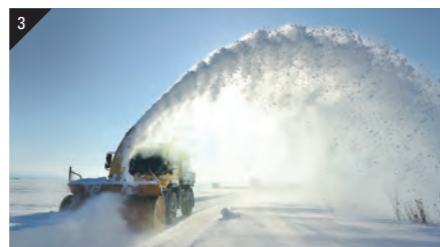
3 A powerful fan equipped to the central snow collector allows long-range snow discharge (over 10m)
