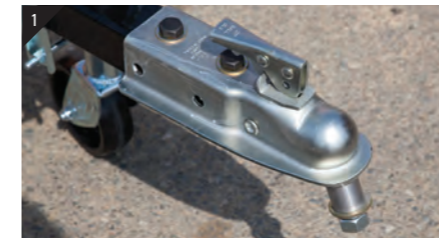
1 Hitch ball and coupling for simple locking and attaching/ detaching
