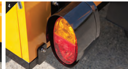
4 Turn signals connected electronically to the main tractor
