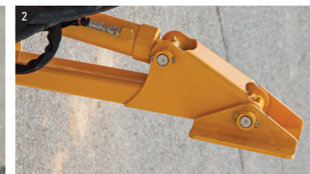
2 Fork-style stabilizer legs are securely supported by the ground, enabling safe and stable working
