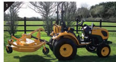
1 Easily attachable to the tractor's rear 3-point hitch
