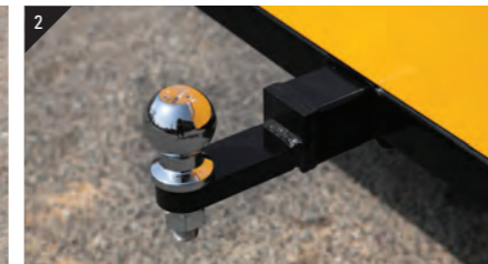
2 Hitch ball on the back of the trailer allows it to be connected to other equipment and trailers can be connected with multiple connections
